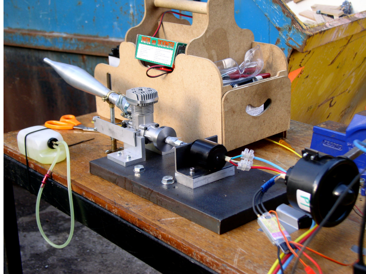
Figure 28 - Fully assembled old Genset test rig
