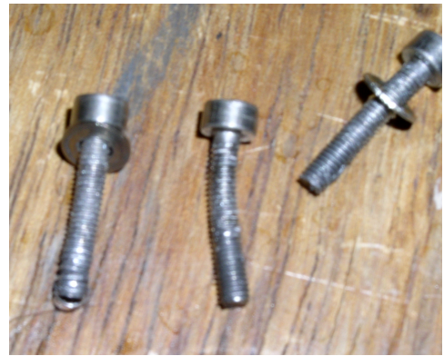
Screws showing stripped aluminium thread
