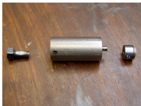
Figure 32 - Shaft, Solid Coupling and flexible coupling
