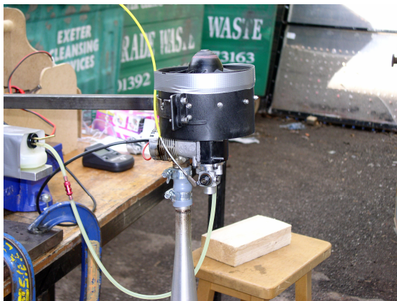
Figure 19 - Vertical Thrust Test Rig (J. Mackenzie-Burrows)
