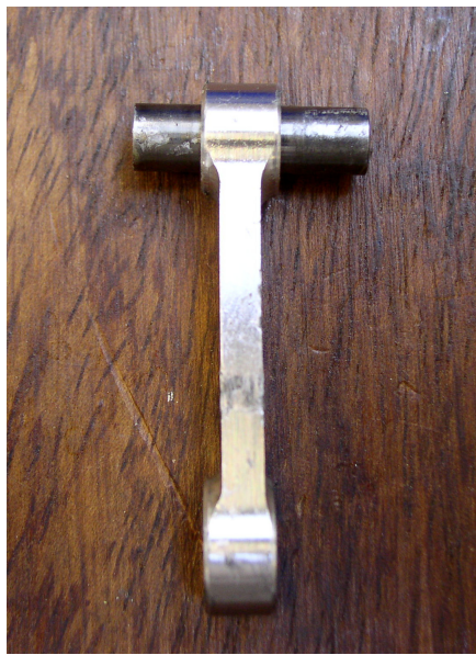
Bent Connecting rod
