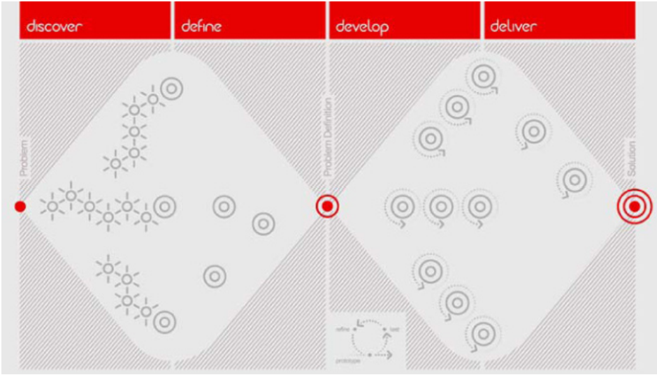
Figure 2.1 – 2 Design Council ‘double diamond’ generic design process model.
