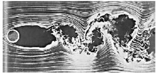
For  $\mathcal{R}e > 10^3$  the von Karman vortex street degenerates into a turbulent wake. The boundary layer in front is still laminar, but separates at an angle of  $81^\circ$
