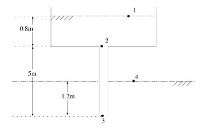
Write down Bernoulli's equation between points 1 (free surface) and 2, between 2 and 3, and between 3 and 4 (free surface again).
