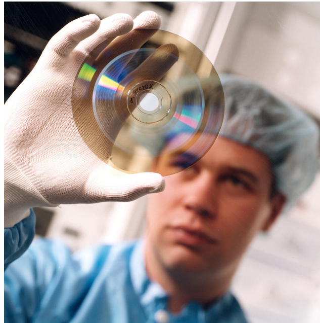
Figure 4.9. A semi-transparent phase-change disc for multi-layer optical recording.
