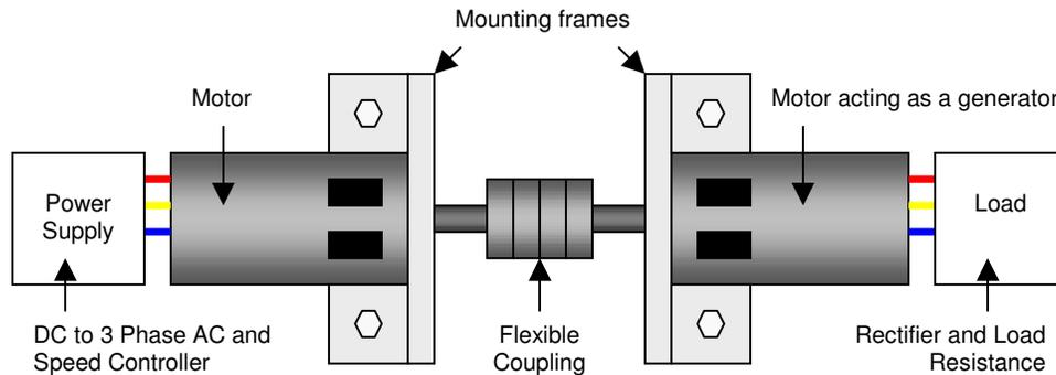
Figure 6.11: Rig for HP 220 Motor Testing
