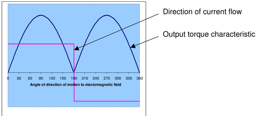
Figure 6.8: Current and torque characteristics of a DC motor
