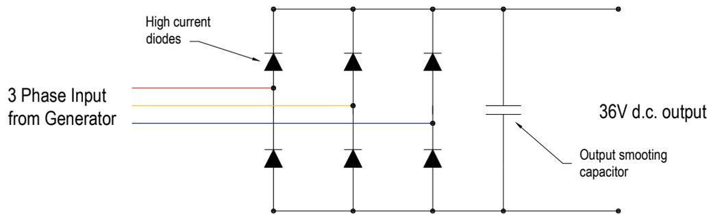
Figure 6.18: 3 phase AC to DC rectifier circuit
