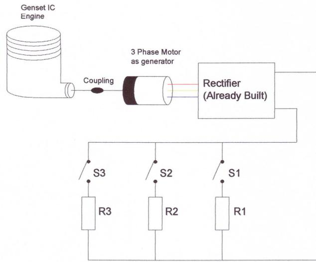
The diagram shows a Genset IC Engine connected via a coupling to a 3 Phase Motor as generator. The generator is connected to a Rectifier (Already Built). The rectifier's output is connected to a three-phase load circuit consisting of three resistors (R1, R2, R3) in parallel, each controlled by a switch (S1, S2, S3).
