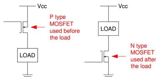
Figure 6.23: Situations to use p and n type MOSFETS
