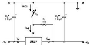
$C_{in}$  is required if regulator is located more than 4 inches from power supply filter. A 1.0  $\mu$ F solid tantalum or 10  $\mu$ F aluminum electrolytic is recommended.
