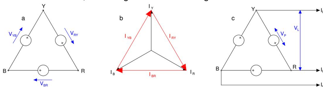
Figure 6.17: Delta Phasors and wiring
