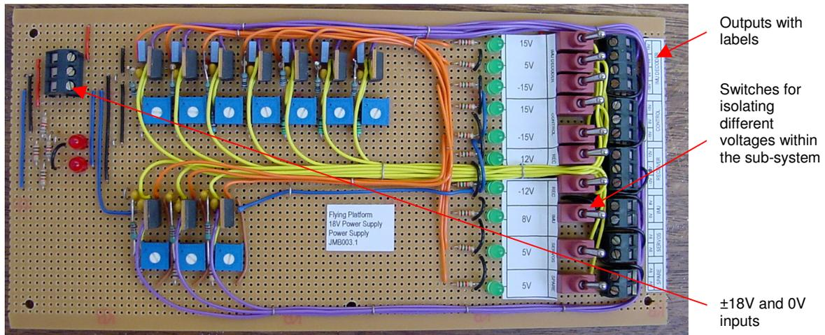
Figure 6.25: Platform power supply with isolation switches for testing purposes only
