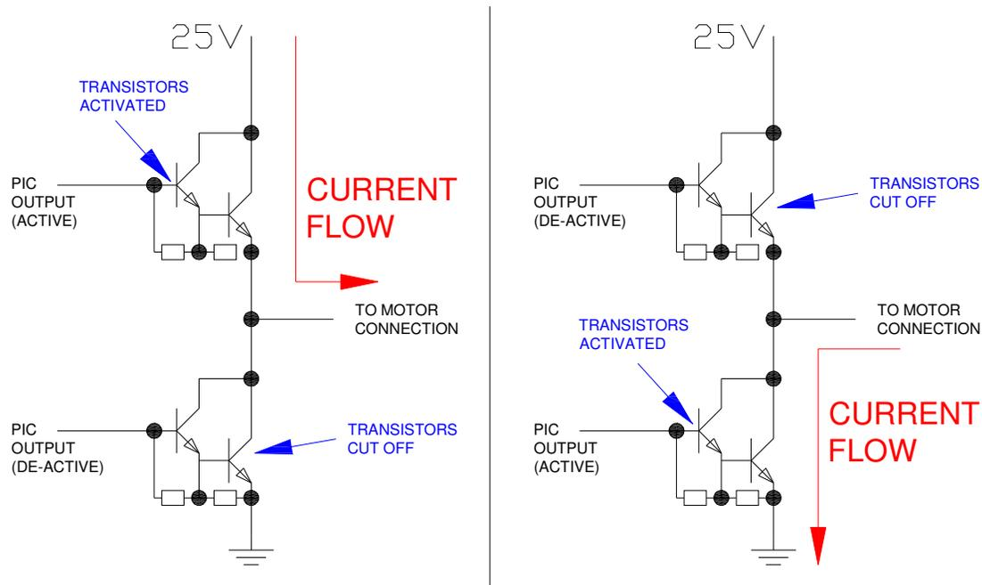
Figure 6.22: The two conditions of current flow either into or out of the motor
