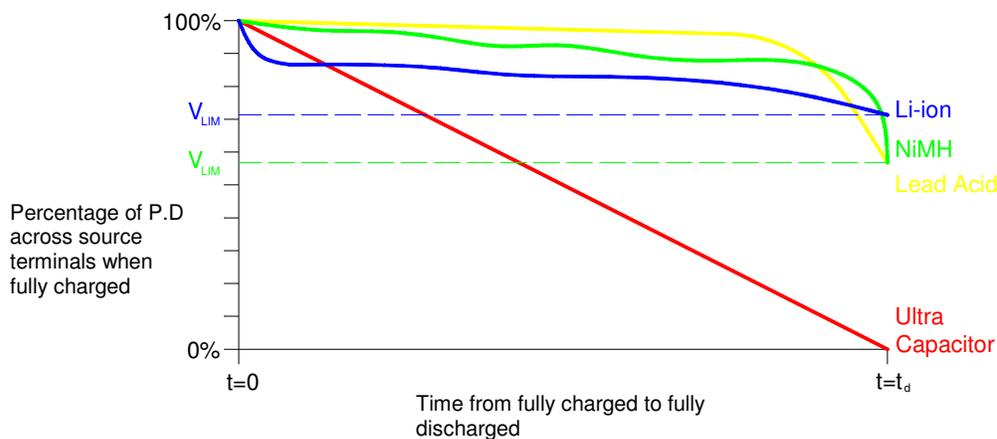
Figure 6.2: Decay trends for different energy storage sources
