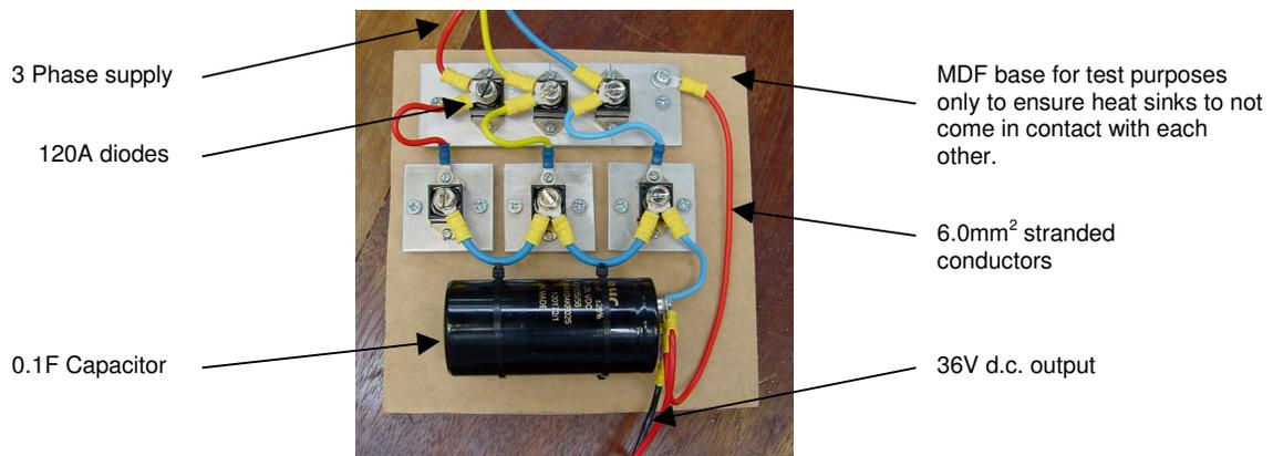
Figure 6.19: Final high current rectifier for testing purposes only
