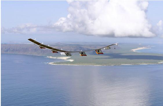
Figure 1.2: NASA's Solar Powered "Helios" Wing during testing [6]
