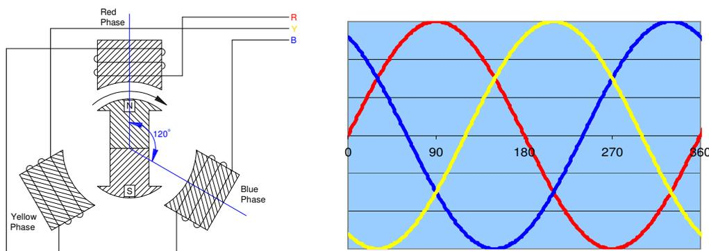
Figure 6.15: A 3 $\Phi$  Generator and output sinusoids
