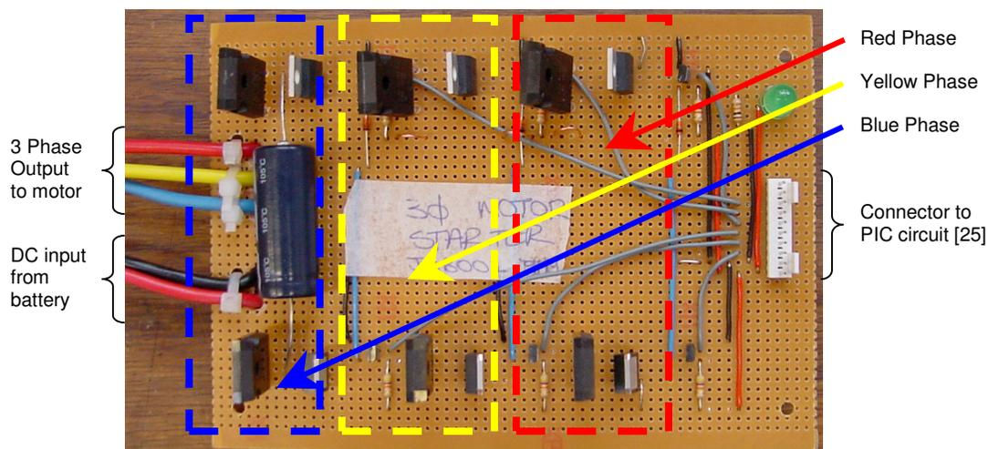
Figure 6.24: Final MOSFET starter circuit
