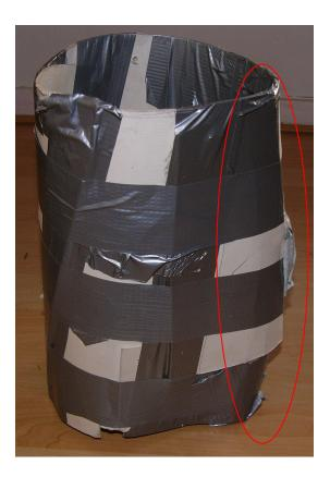
The aim for this duct was to design it on the basis of the Viojett, by keeping the cross sectional area approximately equal, when the engine is taken into account for. There had to be a slot cut into the side of a the ducted fan unit to aid cooling. Energy losses in that area were possible. The red circle denoted the area that binds around the cylinder head. The principle is good though the design lacked the advanced techniques in creating complex shapes.
