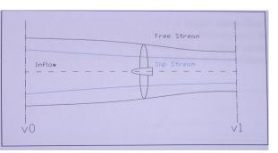
Figure 1 - Flow around a rotor with out duct
