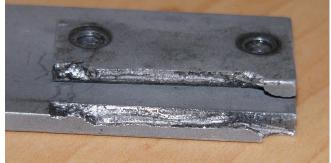
Figure 24 - Crack propagation win the snake arm
