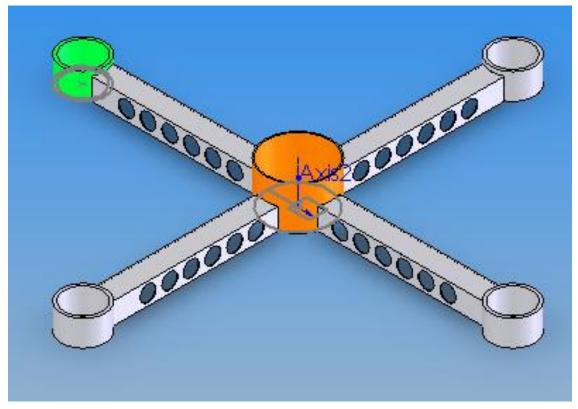
Figure 16 - Box section design
