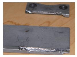
Figure 26 - Snake arm broken parts
