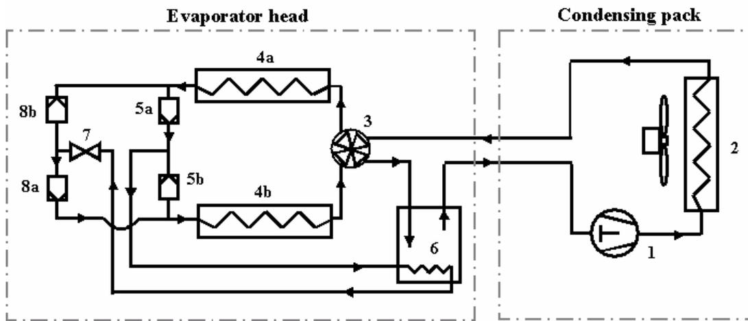
**Figure 1. Refrigeration circuit for recuperative ice generator**
